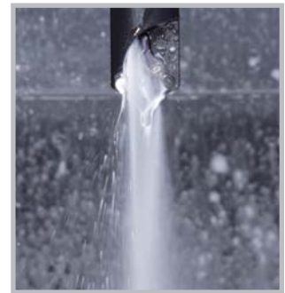
• High pressure coolant can be supplied through center directly to tip of center drill insert.
